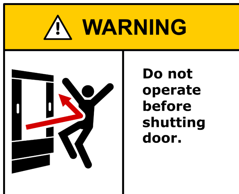
Figure 2.5-2: Safety label for guard doors
