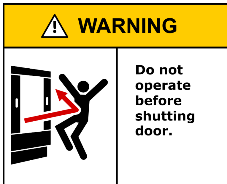
Figure 2.5-2: Safety label for guard doors
