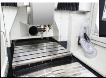
With maximum positional error being less than 5µm and reversal spikes of less than 2µm (when operating at feeds of 8m/min), component manufacturers can achieve high quality machined components delivered in double-quick time.
