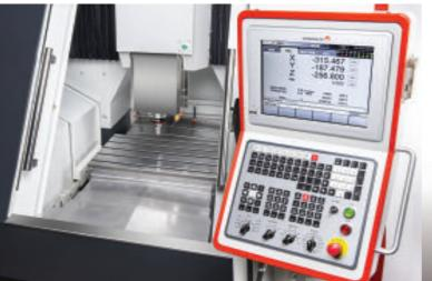
The machine is flexible, powerful and easy-to-use and features a 15" touchscreen control interface, a built-in DXF Reader with integrated DXF Program Editor that supports all programming and editing formats (i.e., Conversational, DXF, ISO/EIA G-Code etc.).
